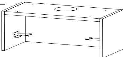
The click-fit angle brackets must be positioned and screwed onto the right and the left side to fit with the suspension element on the side of the extractor hood. (Fig. 3.4).
