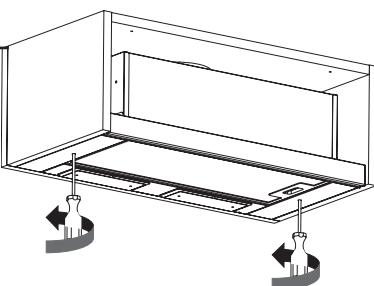
Use a screwdriver to secure the extractor hood in the cabinet. Screw from below using the suspension mechanism as support. (Fig. 3.6).
