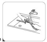
1. To remove the upper spray arm, hold the nut in place and turn the arm counter clockwise.
