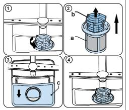
To remove and clean the filter combination, turn it counter clockwise and remove it by lifting it upwards (1).Pull the coarse filter out of the micro filter (2).Then pull and remove the metal filter (3).Rinse the filter with lots of water until it is free of residue. Reassemble the filters. Replace the filter insert, and rotate it clockwise (4).
