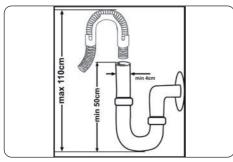
Connect the water drain hose directly to water drain hole or to the sink outlet spigot. This connection should be minimum 50 cm and maximum 110 cm from floor that dishwasher is placed.
