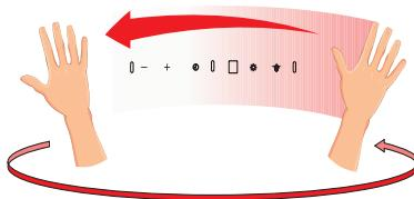
To turn off the fan or reduce fan speed, move your hand from right to left several times in standby mode until the display shows . Move your hand one more time and the appliance will turn off (gesture control will still be active)
