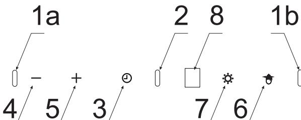
The appliance is fitted with gesture control sensors (1a, 1b, 2) and a display (8).
