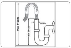
Connect the water drain hose directly to water drain hole or to the sink outlet spigot. This connection should be minimum 50 cm and maximum 110 cm from flor plane.
