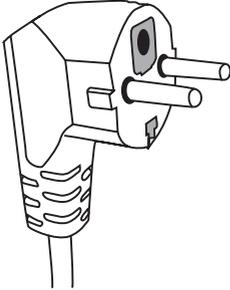
This appliance must be grounded. In the event of a short-circuit, earthing reduces the risk of electric shock. The appliance is equipped with earthing wire with an appropriate plug. The plug should be inserted into a properly installed and grounded outlet.
