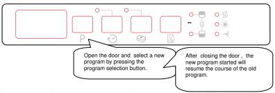
Note: When the door of the machine is opened in order to stop the washing program before it is completed first open the door slightly in order to avoid water spillage.
