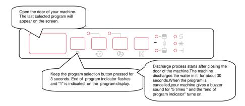
**Note:**When the door of the machine is opened in order to stop the washing program before it is completed first open the door slightly in order to avoid water spillage.
