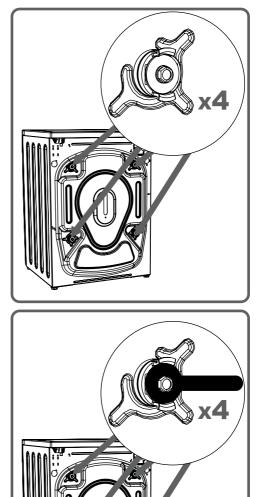
For this reason, transportation safety screws shall be loosened by being rotated in counter-clockwise using an appropriate wrench.
