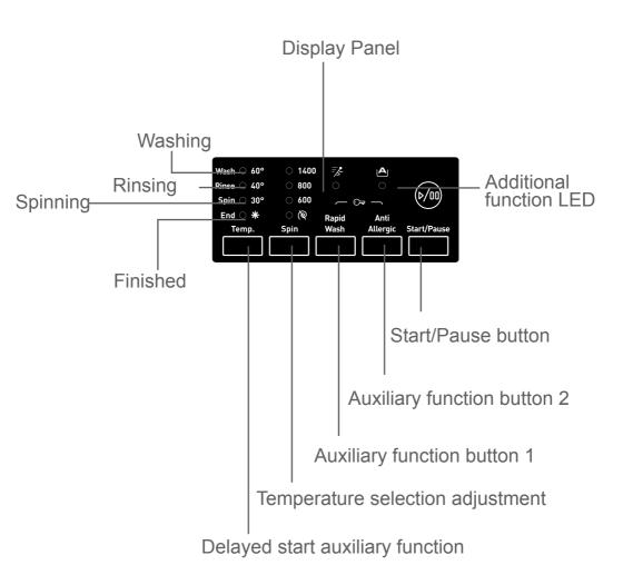
Furthermore, electronic display will warn you by means of led combinations that will turn on its display when a fault occurs on your machine and notify you of the completion of the washing programme by revealing expression of "Finished" on the display as soon as the washing programme you have selected has finished as well.
