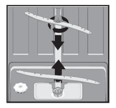
Check whether or not the holes for the upper and lower spray arms are clogged. If there is any clogging, remove the spray arms and clean them under water. You can remove the lower spray arm by pulling it upwards, while the upper spray arm nut can be removed by turning the nut to the left.
