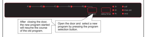
**Note:** When the door of the machine is opened in order to stop the washing program before it is completed, first open the door slightly in order to avoid water spillage.
