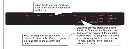
**Note:** When the door of the machine is opened in order to stop the washing program before it is completed, first open the door slightly in order to avoid water spillage.
