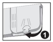
Push the latch to open the detergent container as shown in the image. 1 Detergent pod has level lines inside. It is possible to measure the right detergent amount using these lines. Detergent pod can take totally 40 cm3 detergent. Open the dishwasher detergent and pour into the larger compartment b 25 cm3 if your dishes are heavily soiled or
