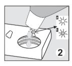
To put rinse aid, remove the rinse aid compartment cap by turning it.1 Fill the rinse aid compartment with rinse aid until the rinse aid level indicator becomes dark; 2 refit the cap and close it by turning it in a way that the nails will correspond to one another. By checking the rinse aid level indicator on the detergent dispenser, you can understand whether or not your machine needs rinse aid. A dark
