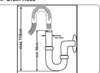
Connect the water drain hose directly to water drain hole or to the sink outlet spigot. This connection should be minimum 50 cm and maximum 110 cm from flor plane.
