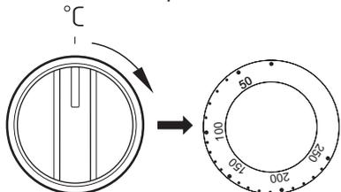
The oven can be switched off by setting both of these knobs to the position "●"/"0".
