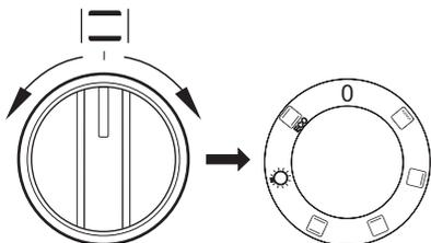
as well as the temperature regulator knob – to set a required function you should turn the knob to the selected position.
