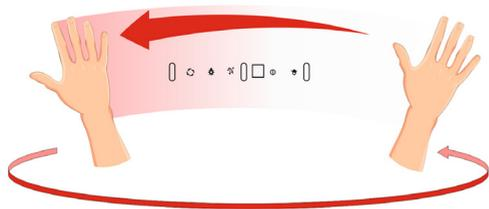
To turn off the fan or reduce fan speed, move your hand from right to left several times in standby mode until the display shows
