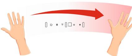
To turn on the fan or increase fan speed, move your hand from left to right several times in standby mode. The display will show the current fan speed after each hand gesture.
