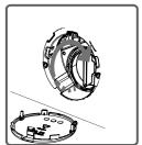
• While closing the pump cover, ensure that the parts on the inner side of the cover to match the holes on the front panel side.
